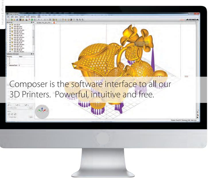
Automatic Support and Part Placement For fast build processing and greater user efficiency
